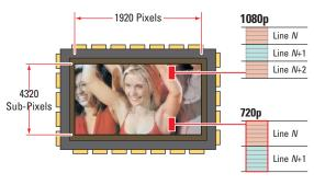
When four vertical sub-pixels are combined per scanning line, the total line count becomes 1080 lines (4320/4 = 1080). So, a 1920 x 1080 image is obtained with a 16:9 aspect ratio.
