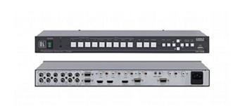
The VP-728 is a 9-input scaler/switcher for analog and digital video, unbalanced stereo, and S/PDIF audio signals. It up- or down-scales any video signal: composite, s-Video (Y/C), component video (YUV), HDMI, computer graphics video and JPEG files to a selectable graphics or HDTV output resolution via identical HDMI or 15-pin HD outputs. It provides glitch-free switching between sources through FTB™ (fade-thru-black) switching technology.
